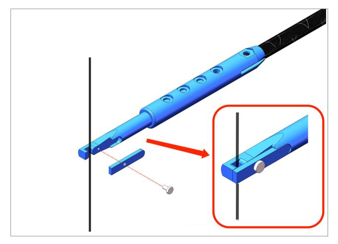
5.Adjust the angle of base, make the opposite angle between imitate arrow shaft and bow string of practise device close to vertical. (Need adjust again after each one time installed.)
