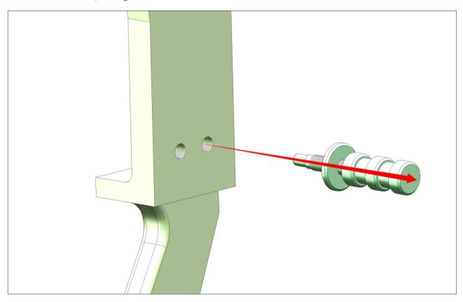
2.Using two 5/16-24 UNF screws to lock the trainer one the riser.
