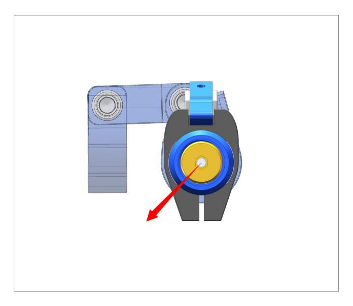
It is 0 ring when anticlockwise revolve to contact shield ring. Clockwise revolve 6 rings is the adjustable max value, then continue revolve maybe caused it damage the seal ring. 2.Please roughly adjust to the below corresponding screw rings first before start to shoot. Please trial shooting from big to small.
