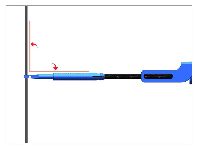
Should do best to adjust the imitate arrow shaft position vertical to the bow string, favour to reduce load of imitate arrow shaft and extend working life.
